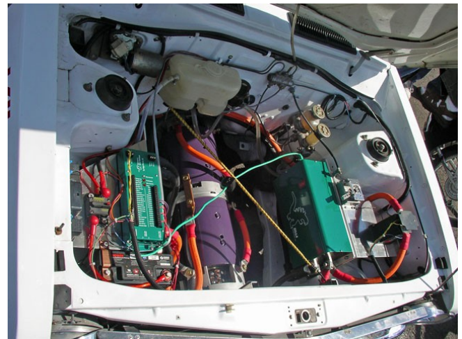
Under the hood of the White Zombie showing the Siamese 8 motors and Zilla controller
